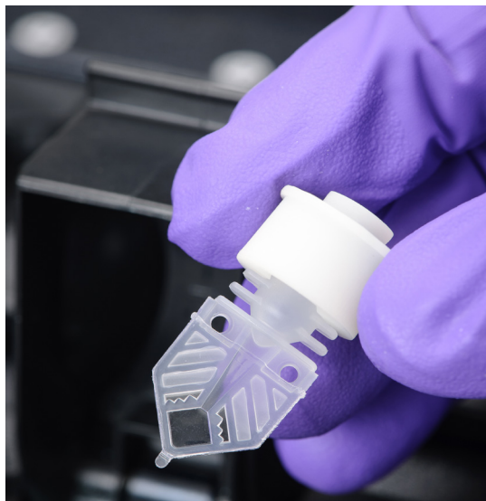
PCR reaction tube with a specialized cap that facilitates liquid handling operations and containment in micro-gravity. Image credit: NASA / Dominic Hart
