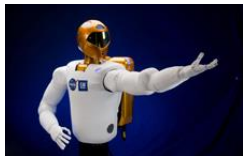
Strategic Objective 1.7, Page 113 The version of Robonaut, R2, currently on the ISS. Robonaut is a dexterous humanoid robot built and designed at NASA Johnson Space Center in Houston, TX. Credit: NASA
