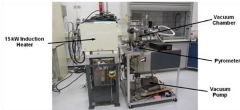
Figure 3-4 Compact Fuel Element Environmental Test facility.
