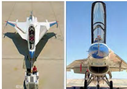
Unique features of the modified F-16XL-2 aircraft included the active suction laminar flow wing glove, the extended left-wing apex, the turbulence diverter (the darker strip along the intersection of the left wing with the forward fuselage), and the shock wave fence under the left wing. (NASA)
