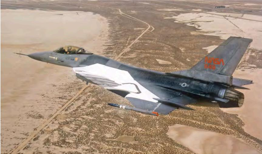
F-16XL-1 with the active suction glove on the left wing that was used for research into supersonic laminar flow control. The grey titanium active suction panel is visible on the inner region of the white wing glove. The passive outer leading edge of the wing glove is painted black in the region where a liquid-crystal sensor array was located. A video camera in the wingtip pod was used to record the liquid-crystal patterns. (NASA)
