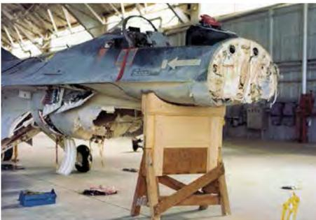
The damaged fuselage of the third Full-Scale Development F-16A (75-0747) following its emergency landing and nose gear collapse on Rogers Dry Lake, October 5, 1980. (NASA photograph via Tom Grindle)
