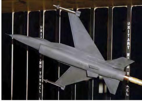
A wind tunnel test model of a modified F-16 fuselage fitted with a forward-swept wing mounted in the NASA Langley Unitary Plan Wind Tunnel in 1980. (NASA)
