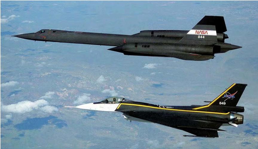
F-16XL-1 was used for sonic boom probing tests with the NASA SR-71. The F-16XL's speed brakes are extended in this photo taken at subsonic speed; however, the F-16XL had a difficult time maintaining formation with the SR-71 above Mach 1.5. (NASA)
