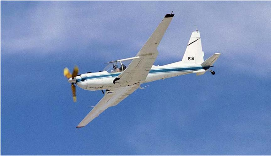
A NASA Lockheed YO-3A was used to measure the sonic boom signatures emanating from a Lockheed SR-71 flying at supersonic speed at much higher altitudes. (NASA)
