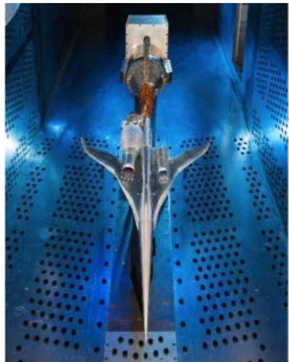
Figure 22: Wind tunnel design validation of sonic boom signatures, inlet, and nozzle effects.
