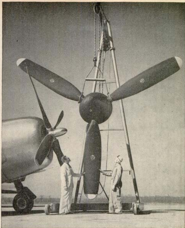
Not a last look, insists the author. Six of these 19-foot propellers pull the world's largest landplane, the XC-99, through the air. Blades' pitch can be reversed to brake landing run
