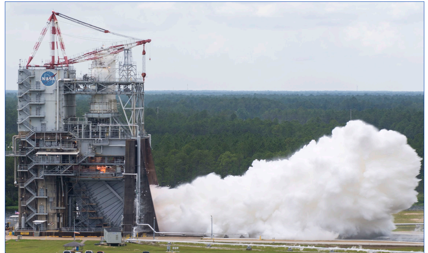
Stennis Space Center operators conduct a successful initial test of the Aerojet Rocketdyne AR-22 rocket engine on the A-1 Test Stand on June 12.
