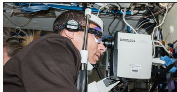
As part of the Ocular Health Study, a crewmember has his eye imaged using Optical Coherence Tomography (OCT).
