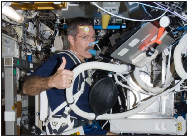
An ISS crewmember cycles on the ergometer while performing a VO 2 max test. This method of testing involves capturing all of the expired 'breath' which is then analyzed.
