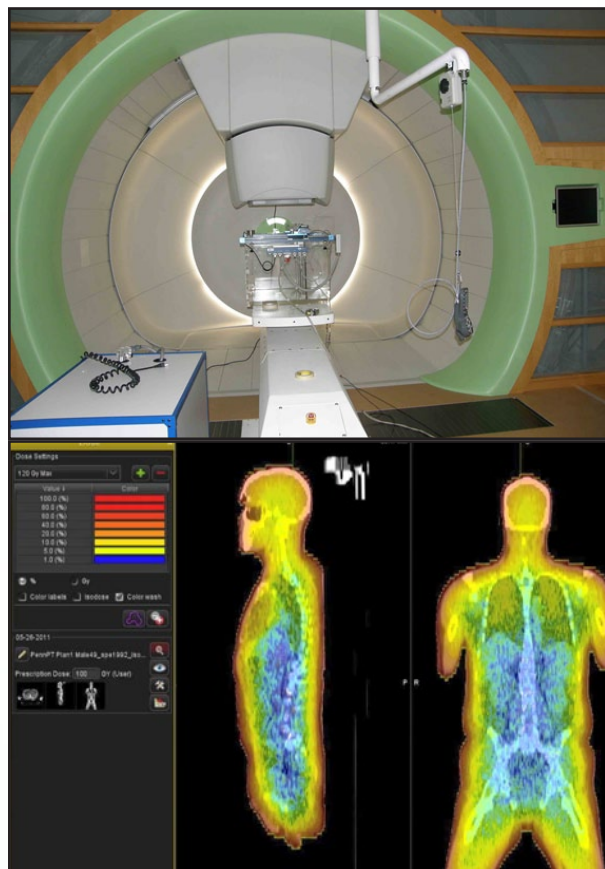
CARR Investigators utilized the University of Pennsylvania Proton Facility for studies on the effects of SPEs (top photo). Special tools utilize magnetic resonance imaging (MRIs) to study how SPE dose distribution varies based on a person's unique physiology (bottom).
