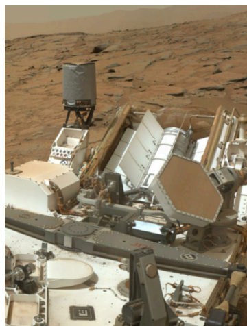
The Curiosity rover took this self portrait on the surface of Mars, with its MMRTG power source visible at the rear.
