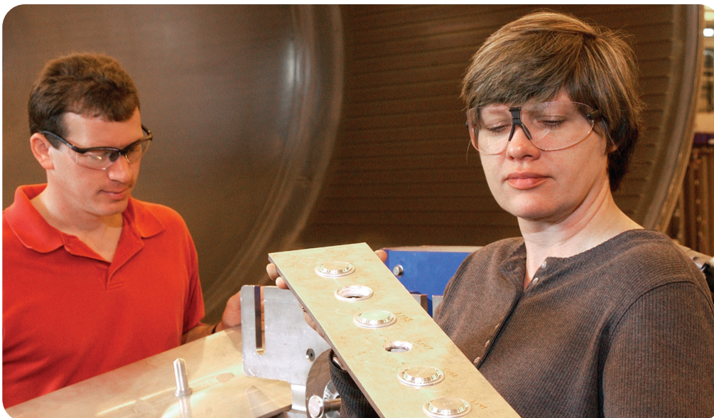
NASA materials engineer Carolyn Russell inspects sample weld plugs on a piece of light weight aluminum.
