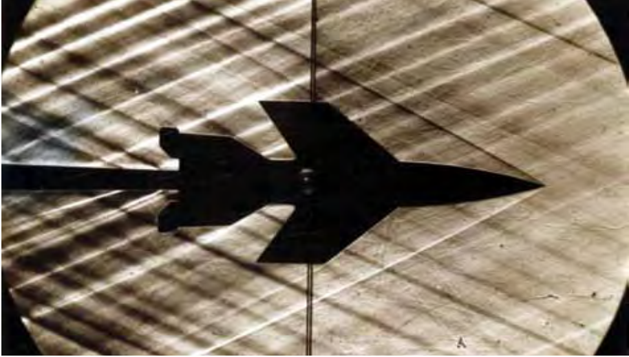
Figure 6: Shock wave pattern formed at Mach 2.5 by the A4 V12/c, a swept-wing variant of the A-4 (V-2) missile, 1940. Richard Lehnert, "Bericht über Dreikomponentenmessungen mit den Gleitermodellen A4 V12/a und A4 V12/c," Archiv Nr 66/34 (Peenemünde: Heeres-Versuchsstelle, 27 November 1940), Box 674, "C10/V-2/History" file, National Museum of the United States Air Force, Wright-Patterson Air Force Base, Ohio
