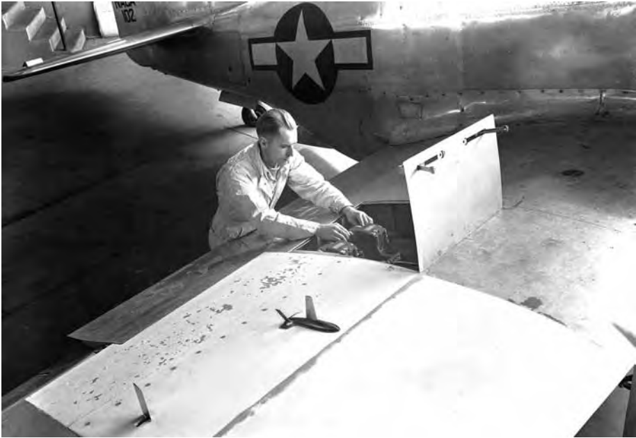
Figure 3: A technician readies the recording instrumentation of a P-51D Mustang modified for wing-flow transonic research. The test model (an XS-1 shape with a swept horizontal tail) is at midspan, with mechanical linkages connecting it to the instrumentation installed within the modified gun bay. NASA Image L-46802
