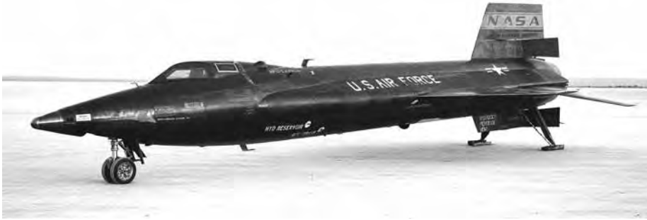
Figure 17: North American X-15 Mach 6+ hypersonic transatmospheric research aircraft. NASA Image E-7411
