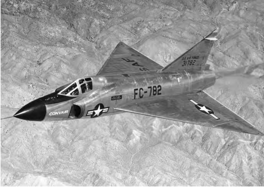
Figure 13: The Convair YF-102 Delta Dagger interceptor, as originally flown without area ruling. Convair
