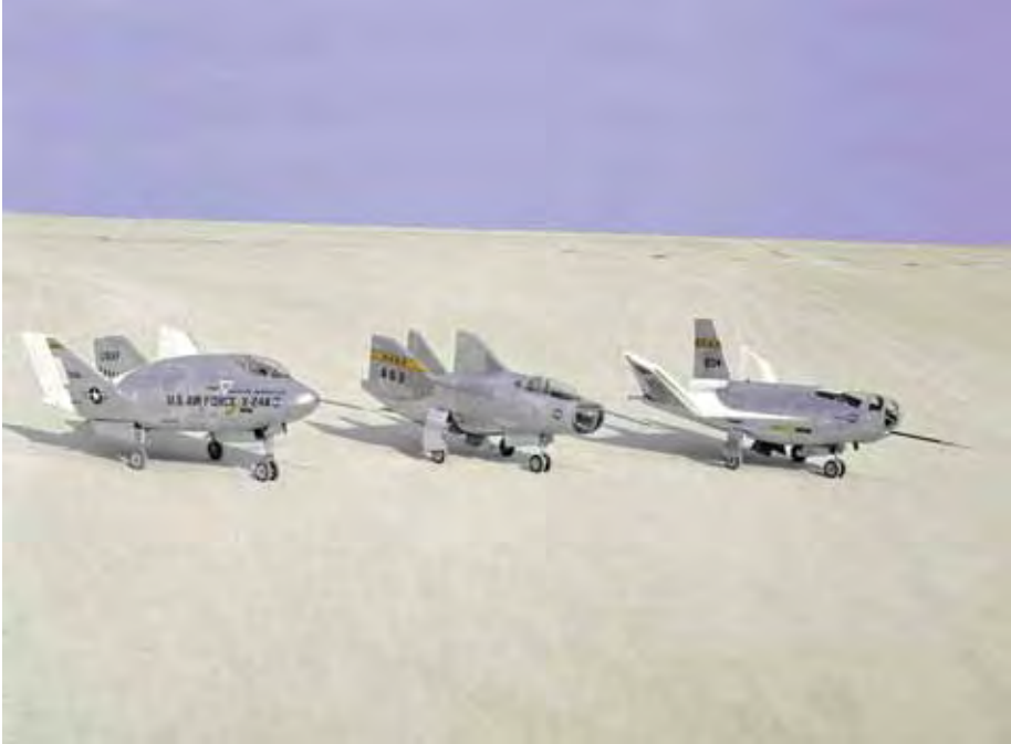
Figure 5: The wingless lifting body aircraft sitting on Rogers Dry Lake at what is now NASA's DFRC, Edwards, California. From left to right: the U.S. Air Force X-24A, FRC M2-F3, and Langley HL-10. The lifting body aircraft studied the feasibility of maneuvering and landing an aerodynamic craft designed for reentry from space. These lifting bodies were air-launched by a B-52 mother ship; they then flew powered by their own rocket engines before making an unpowered approach and landing. They helped validate the concept that a space shuttle could make accurate landings without power. The X-24A flew from 17 April 1969 to 4 June 1971. The M2-F3 flew from 2 June 1970 to 21 December 1971. The HL-10 flew from 22 December 1966 to 17 July 1970 and logged the highest and fastest records in the lifting body program. NASA Image EC69-2358
