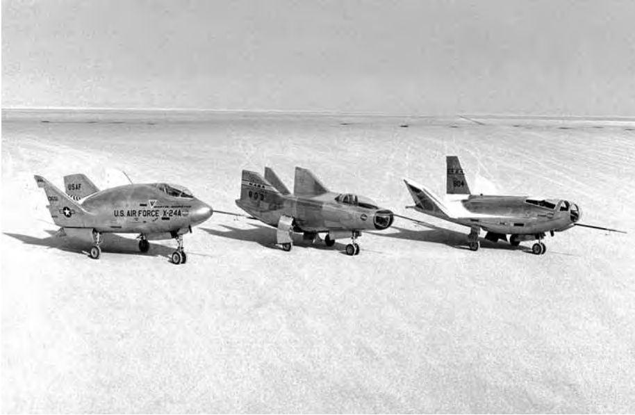
Figure 19: The NASA-Air Force lifting body family in 1969. From left to right are the Martin X-24A, Northrop M2-F3, and Northrop HL-10. The X-24 constituted an Air Force initiative and later spawned the X-24B, which had a much higher fineness ratio. The M2-F3 and HL-10 were “rival” concepts, the former a modified half-cone derived by Ames, the latter a fattened delta derived by Langley. NASA Image E-21093
