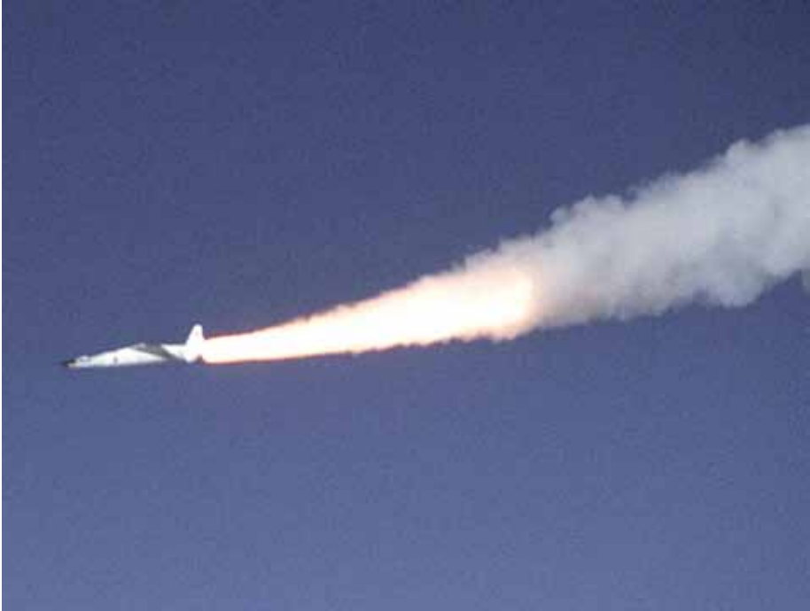
Figure 23: The third X-43A accelerates to Mach 9.7 prior to release from its Pegasus booster, 16 November 2004, following air-launch over the Pacific Ocean from its Boeing NB-52B mother ship. NASA Image EC04-0325-37
