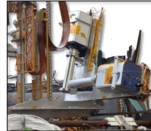
Two commercial versions of MSolo (Open Ion and Cross-Beam sensor configurations) in test configuration
