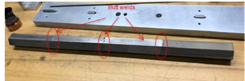
Butt weld development of stainless steel NTREES N-19 article: May possibly use as an additional fit-up article for NTREES testing
