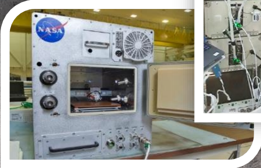
Refabricator is the first integrated 3D printer and recycler in space and currently aboard ISS
