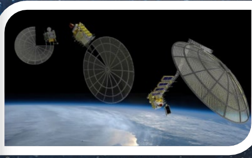
Made In Space validated additive manufacturing and robotic assembly with a future mission, Archinaut
