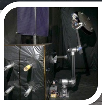
Made In Space validated additive manufacturing and robotic assembly with a future mission, Archinaut
