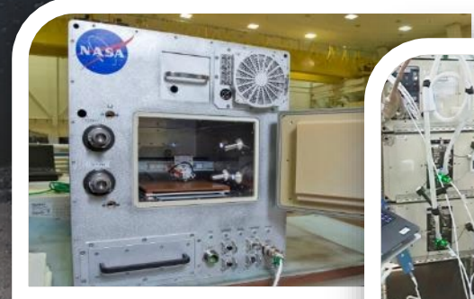
Refabricator is the first integrated 3D printer and recycler in space and aboard ISS. However it experienced a failure with the novel recycler filament extrusion bonding system in 2019. Additional bonder testing will be performed prior to decommissioning. The Refabricator was able to successfully manufacture a tensile specimen on the ISS in Feb. 2020 which will be brought back soon for further testing and evaluation aboard SpaceX-20 in April 2020
