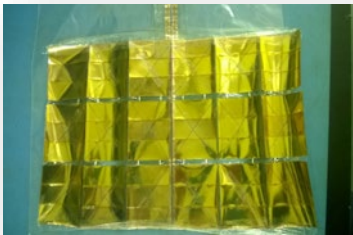
MSFC LISA-T (Lightweight Integrated Solar Array and Transceiver) self-unfolding system worked well. Investigating flight system for cubesat. Flying various elements on MISSE 10.
