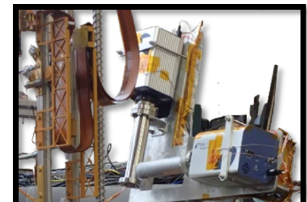
Two commercial versions of MSolo (Open Ion and Cross-Beam sensor configurations) in test configuration
