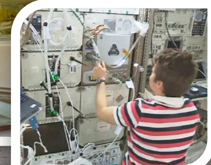
Refabricator is the first integrated 3D printer and recycler in space and aboard ISS. However it experienced a failure with the novel recycler filament extrusion bonding system in 2019. Additional bonder testing will be performed prior to decommissioning. The Refabricator was able to successfully manufacture a tensile specimen on the ISS in Feb. 2020 which will be brought back soon for further testing and evaluation aboard SpaceX-20 in April 2020
