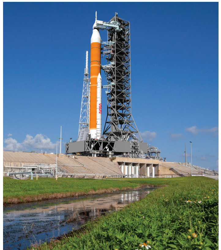
An artist rendering of the Space Launch System (SLS) Block 1B atop the mobile launcher 2 at Kennedy Space Center's Launch Pad 39B in Florida. The SLS Block 1B configuration will be used to send cargo to the Moon under NASA's Artemis program. Photo credit: NASA/David Zeiters
