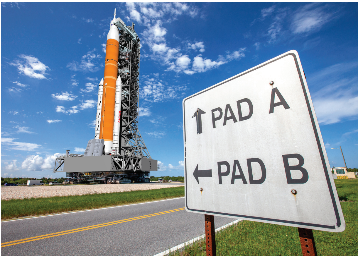
An artist rendering of crawler-transporter 2, with the mobile launcher 2 and Space Launch System (SLS) Block 1B atop, as it makes its way to Launch Pad 39B in preparation for liftoff. The SLS Block 1B configuration will be used to send cargo to the Moon under NASA's Artemis program. Photo credit: NASA/David Zeiters
