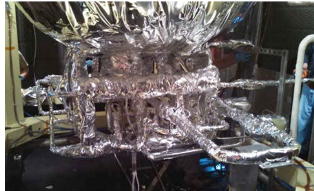
Low emissivity wrap completed
