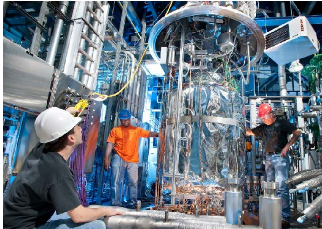
Workers in the Small Multipurpose Research Facility at GRC conduct liquid hydrogen reduced boil-off testing
