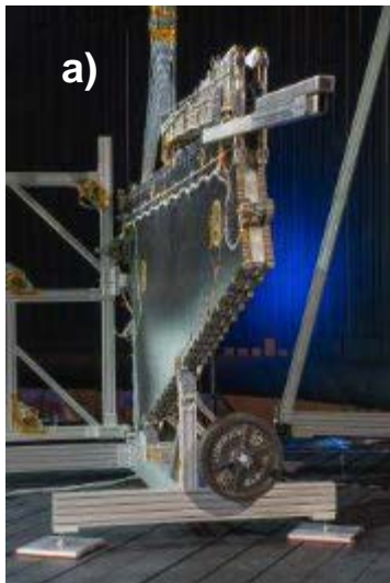
Deployment testing in thermal vacuum chamber
