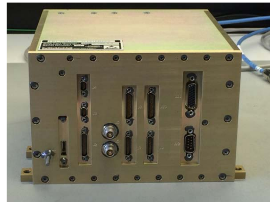
Controller Electronics Engineering Development Unit
