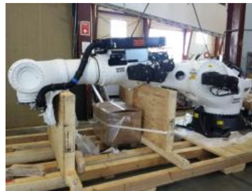
LaRC Automated Fiber Placement (AFP) system at the vendor facility
