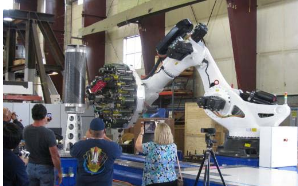
LaRC Automated Fiber Placement (AFP) system at the vendor facility
