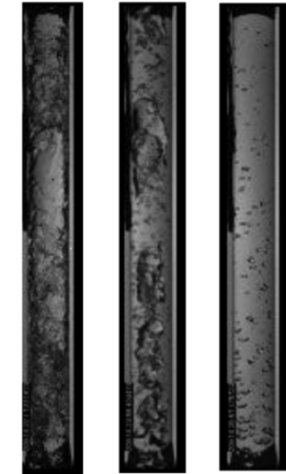
Slight Glass during Line Chillardown
