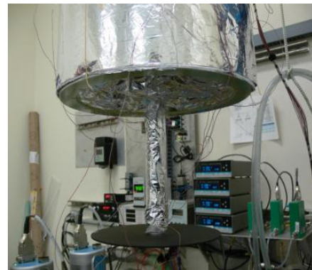
(MLI) Penetration Heat Leak Study
