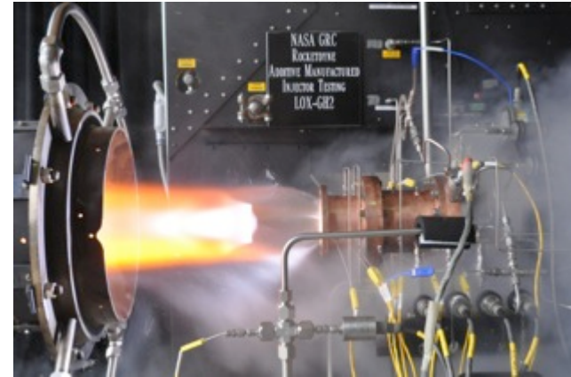
Aerojet Rocketdyne additive manufactured injector test in RCL Cell 32, June 2013
