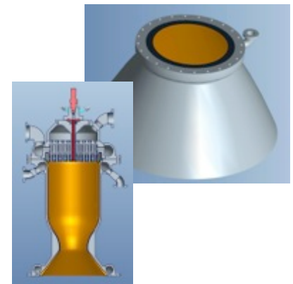
Copper Alloy, Regeneratively Cooled Chamber and Nozzle
