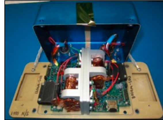
Radiation Environment Monitors measured radiation inside Orion when it passes through Van Allen belts.
