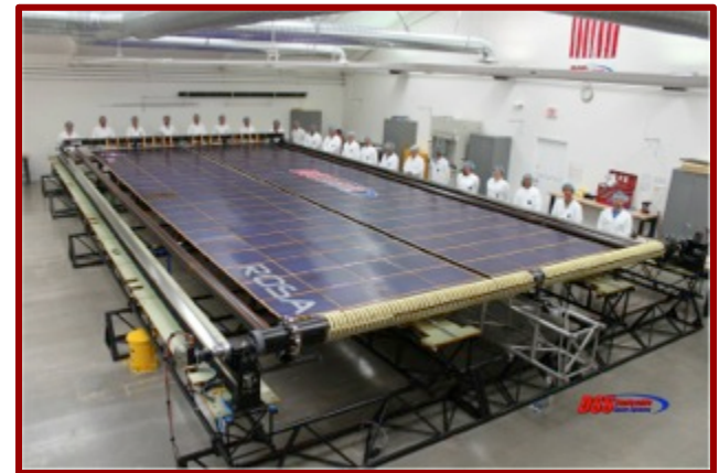
DSS ROSA Engineering Development Unit (EDU) employs strain-energy deployed STEM (storable tubular extendable member) booms to reduce mechanical complexity, parts & deployer recurring costs.
