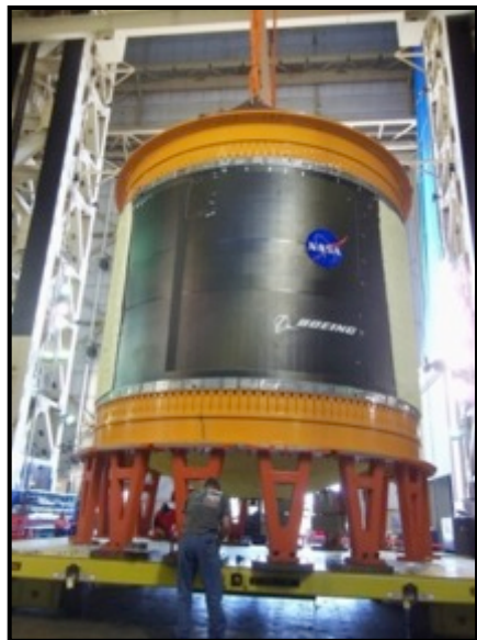
5.5m diameter composite cryotank
