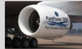
P&W PurePower 1000G Geared Turbofan
