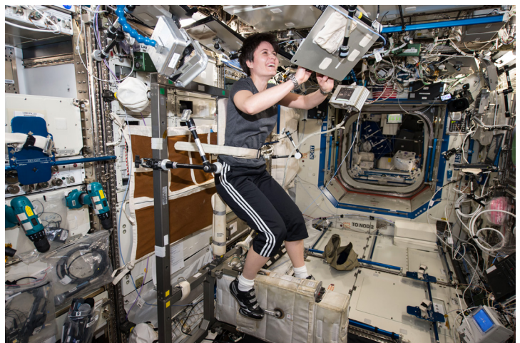
European Space Agency astronaut Samanta Cristoforetti exercises on the space station's Cycle Ergometer with Vibration Isolation and Stabilization (CEVIS). As astronauts sweat and generate carbon dioxide, the ECLSS system recycles both into usable water and breathable air. (NASA)
