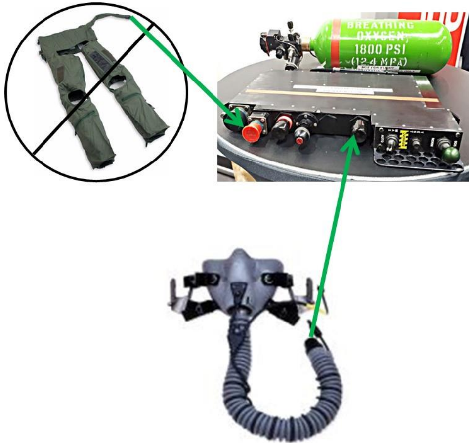
Figure 6.7. G-suit (left), black electronic regulator [below a BOS bottle] (right), and mask (bottom). Both G-suit and mask connect to the BRAG [note that the mask shown is not an F-35 mask; the figure only depicts proper system connection locations].
