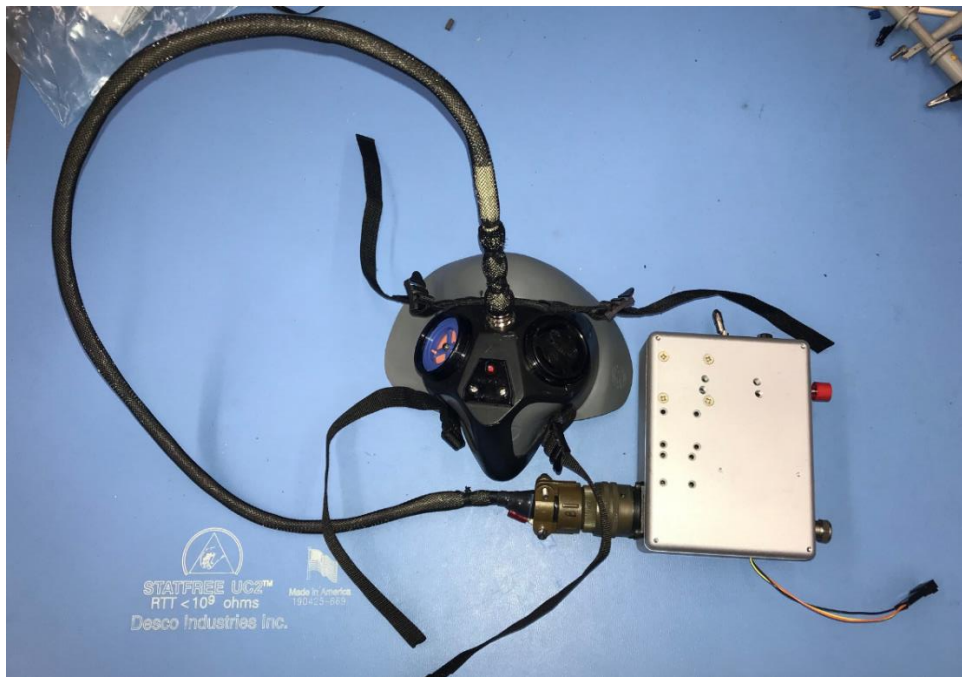
Figure 2 Photo Showing External Power Supply and Connecting Cable
