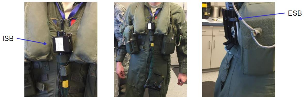
Figure 4.1. Locations of the VigilOX Inhalation Sensor Block (ISB) and Exhalation Sensor Block (ESB) on the Pilot
