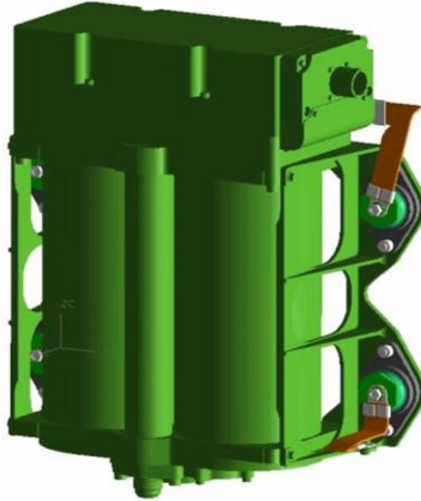
A.11 F-35 Lightning II Figure A-11. F-35 On-Board Oxygen Generating System.
