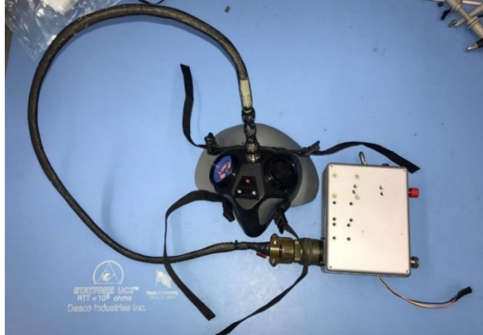
Figure 9.1. Photograph of IMCWS Configuration Showing Mask, Cable, and External Power Supply Box
