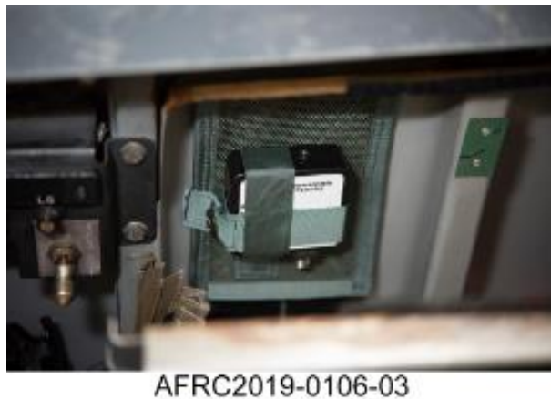
Figure 1.16. MadgeTech Pressure Sensor Mounted in Cockpit Map Case to Measure Cabin Pressure for PBA Flights After Flight 60, Both USN and USAF Configurations
