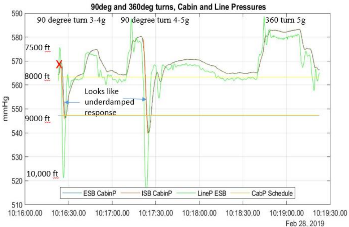
Figure 6.9.2.4. Shows 2 Cabin Pressure Dips the prominent one being a nearly 2,000 ft pressure excursion, and registering over then under the 8,000 ft prescribed isobaric pressure
