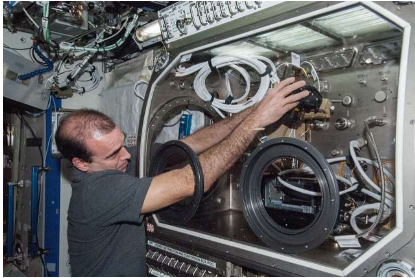
NASA astronaut Rick Mastracchio sets up the Microgravity Science Glovebox (MSG) for a combustion experiment in February 2014.
