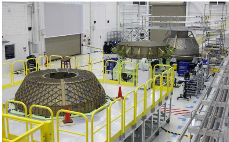
Figure 9. Boeing CST-100 Structural Test Article Being Assembled at KSC
