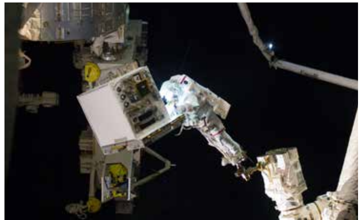
Figure 4. NASA's Robotic Refueling Mission system being installed on the International Space Station. Source: NASA.
