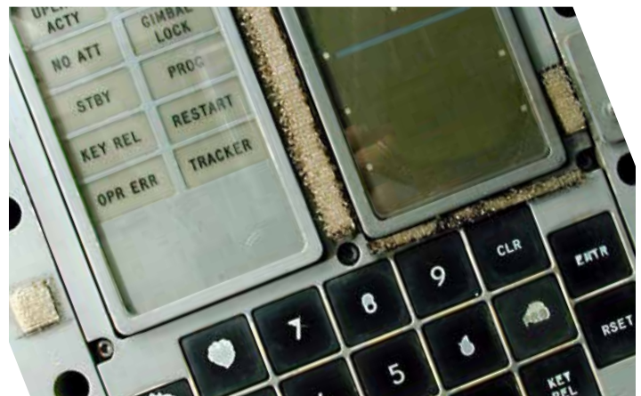
Figure 1. The Display and Keyboard (DSKY) mounted in the Main Display Console of Apollo 13's Command Module "Odyssey." The DSKY is connected to the Apollo Guidance Computer. Source: Bruce Yarbrow/Smithsonian Institution.
