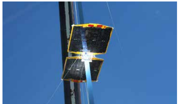
Figure 18. The University of Michigan's MClimber, an entrant into the 2006 Space Elevator Games - Power Beaming competition. The system successfully reached 50-meter mark. Source: Dustin Sensiba.
