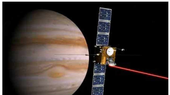
Figure 20. Artist's impression of a laser communications system employed near Jupiter. Source: NASA.
