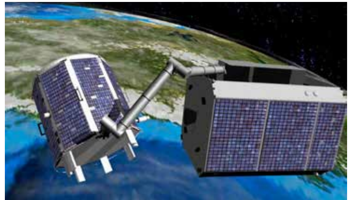
Figure 6. Artist impression of the servicer turning the client for docking maneuver. Source: SpaceTech GmbH.
