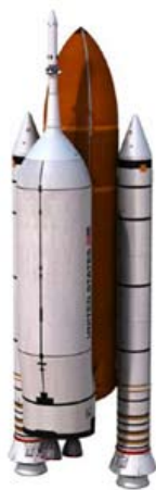
Figure 5.2.2-2. Shuttle-Derived Sidemount Launcher. Source: NASA
