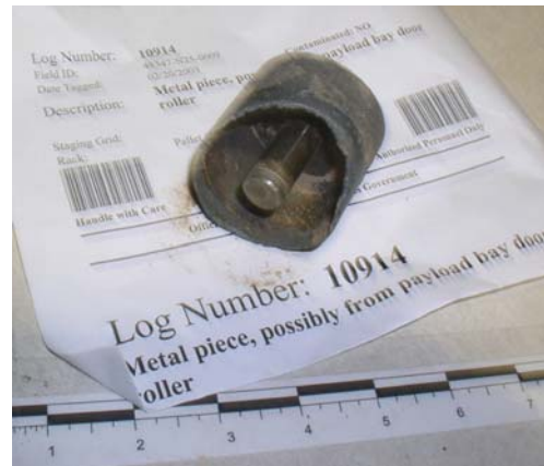
Figure 2.1-53. Recovered payload cylinder bay door roller with inner material absent and Inconel sleeve remaining. [Columbia Reconstruction Database, debris item no. 10914]
