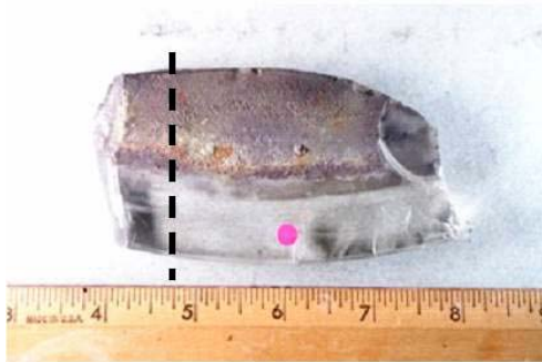
Figure 2.4-60. Window fragment removed from the thermal pane frame from Window 8. The black dashed line denotes the sectioning plane. The red dot was used to indicate the outward face of the pane.
