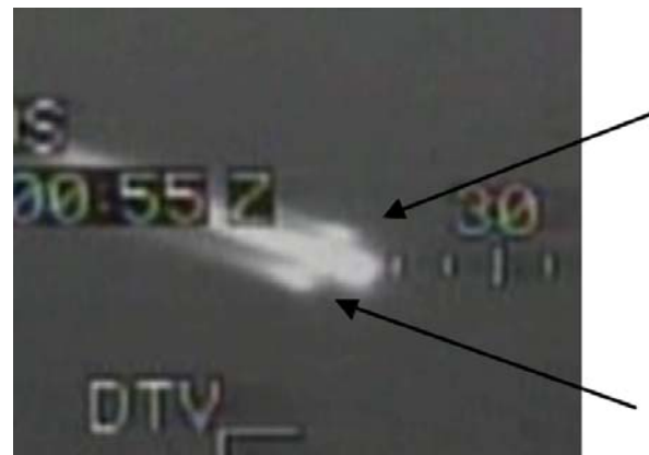
Figure 1.1-30. Video frame from the Apache video at GMT 14:00:55 (EI+1006) showing two similar luminosity objects separating from the forebody.
