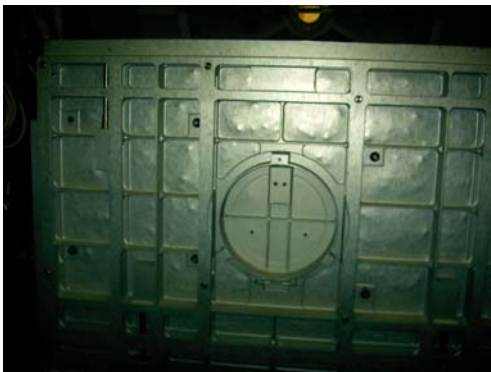
Figure 2.1-37. Lower surface of the lithium hydroxide door, facing the lower equipment bay (mockup).
