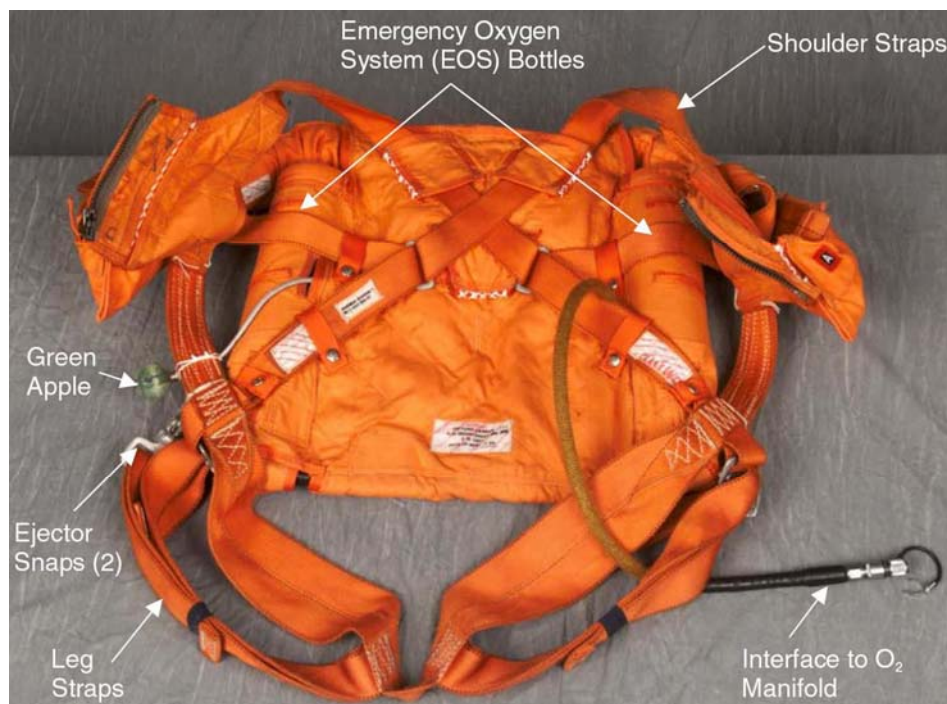
Figure 3.2-11. Example of parachute harness.
