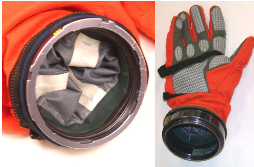
Figure 3.2-25. Examples of intact suit-side (left) and glove-side (right) glove disconnects.
