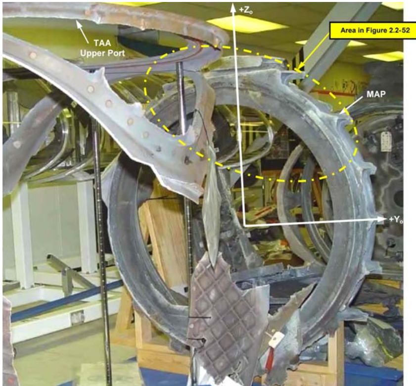
Figure 2.2-51. Tunnel adapter assembly and the manufacturing access panel debris, view looking forward at "B" hatch opening.
