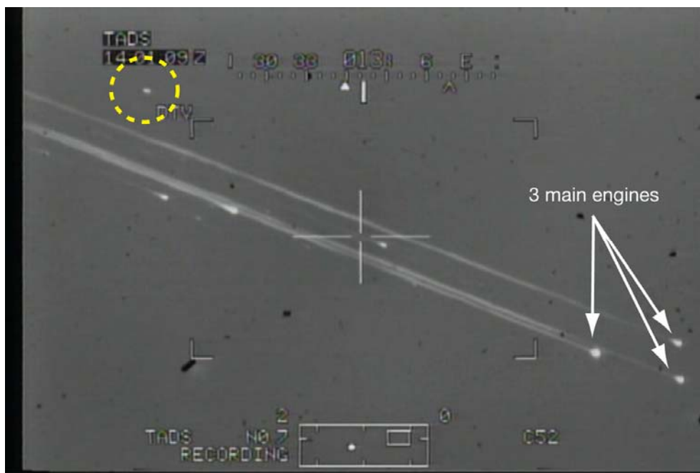
Figure 1.2-48. Image is from the Apache video. Dotted circle indicates area where crew module debris is last visible. The three points in the lower right are the three main engines.
