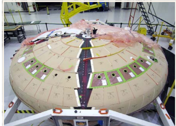
FIGURE 6. Avcoat Block Heat Shield Installation Underway
