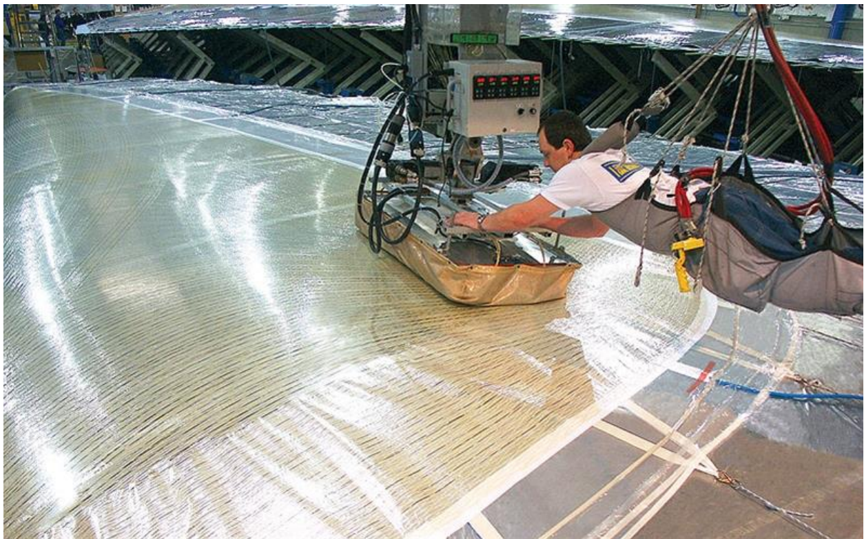
Figure V.B.6. Northsail 3DL® Process. The 3DL® process molds the entire sail over a three-dimensional mold.
