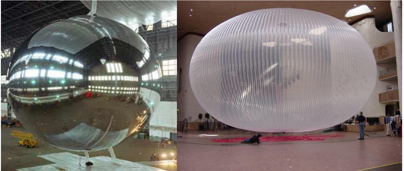
Figure V.B.3. Typical “gore” pattern sections used in most scientific balloons
