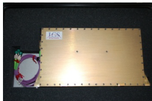
PPM laser transmitter with 10% efficiency (TRL-6)
