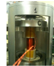
JPL hybrid active/passive strut with 50 dB isolation at 5 Hz (TRL 4)
