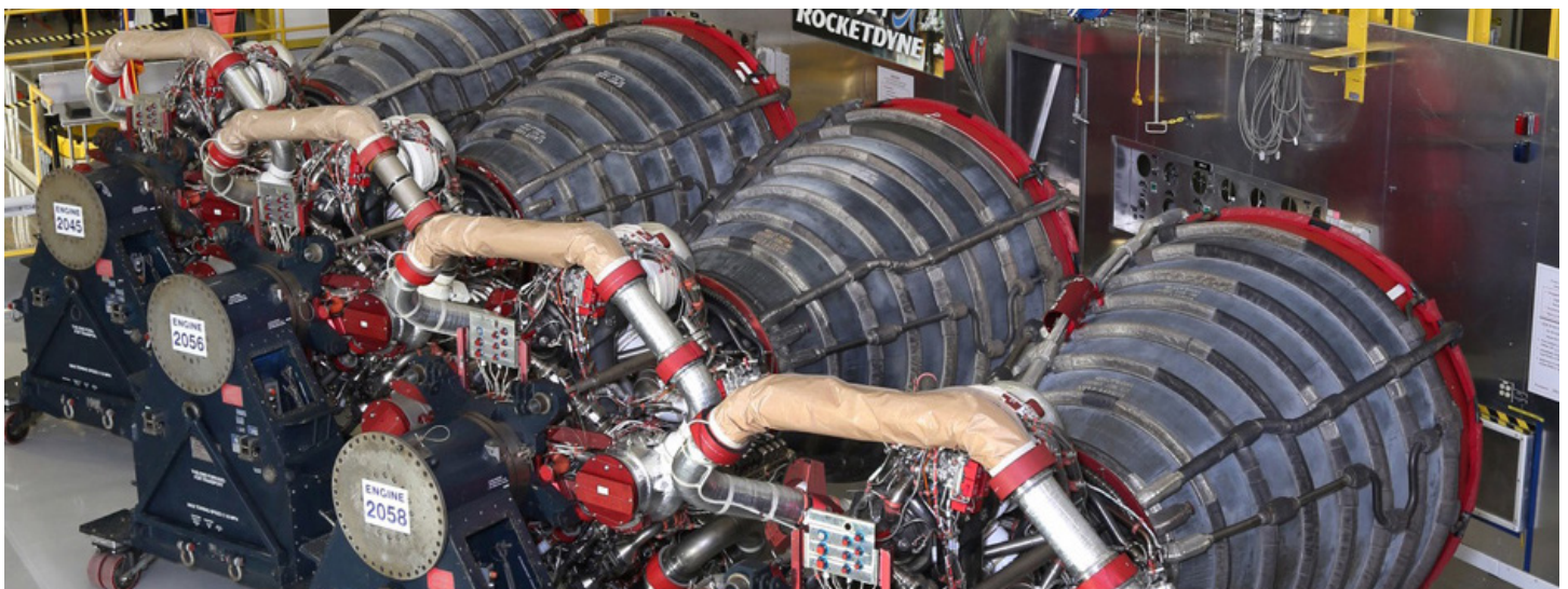
The four RS-25 engines that will power SLS for its first flight.
