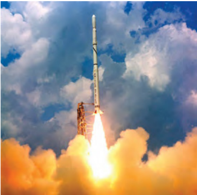
Four-stage, solid propellant Scout rocket.
