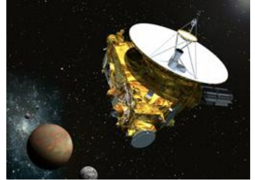
Figure 1. An artist’s rendering of the New Horizons spacecraft as it approaches Pluto. The prominent 2.1-meter dish antenna is used to communicate with Earth from up to 7.5 billion kilometers away. (Image credit: JHUAPL/SwRI)
