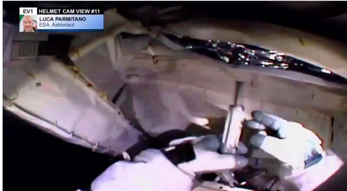
Astronaut Luca Parmitano uses the zip-tie cutter during a spacewalk to repair the Alpha Magnetic Spectrometer on Nov. 15, 2019. Image Credit: NASA
