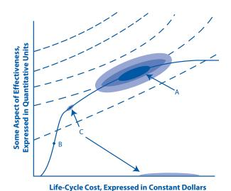
FIGURE 4.4-3 A Quantitative Objective Function, Dependent on Life Cycle Cost and All Aspects of Effectiveness
