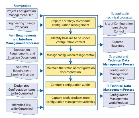
FIGURE 6.5-1 Configuration Management Process
