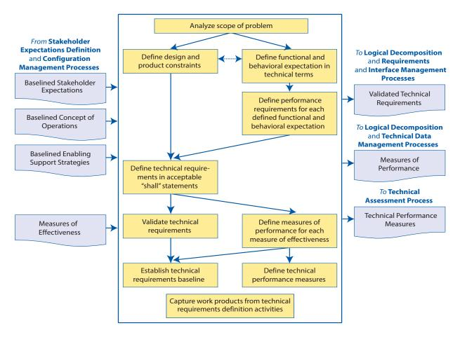
FIGURE 4.2-1 Technical Requirements Definition Process
