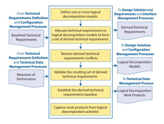
FIGURE 4.3-1 Logical Decomposition Process
