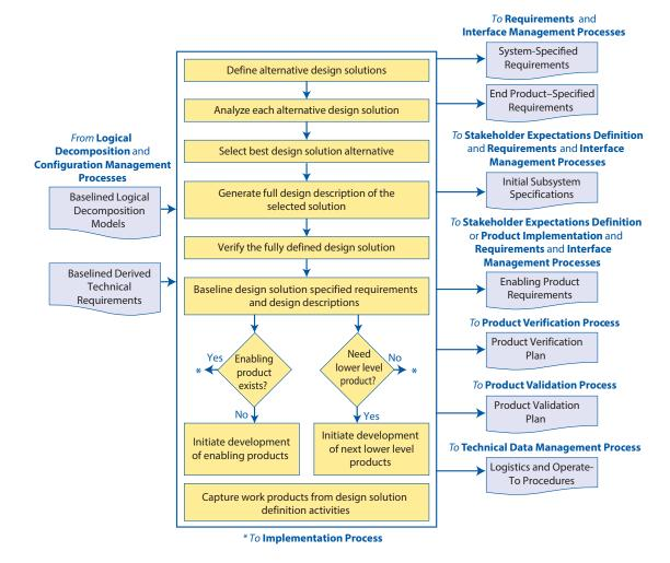
FIGURE 4.4-1 Design Solution Definition Process
