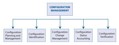
FIGURE 6.5-2 Five Elements of Configuration Management
