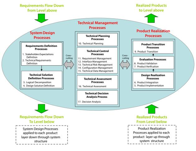
FIGURE 2.1-1 The Systems Engineering Engine (NPR 7123.1)
