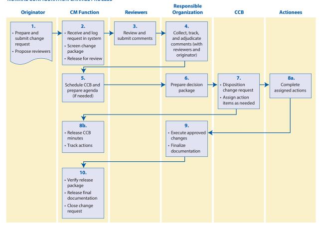
FIGURE 6.5-4 Typical Change Control Process
