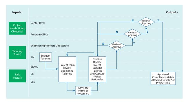
FIGURE 3.11-1 Notional Space Flight Products Tailoring Process
