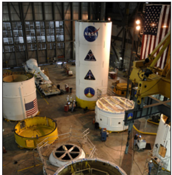
The upper stage simulator segments are ready for stacking in Kennedy Space Center's Vehicle Assembly Building.
