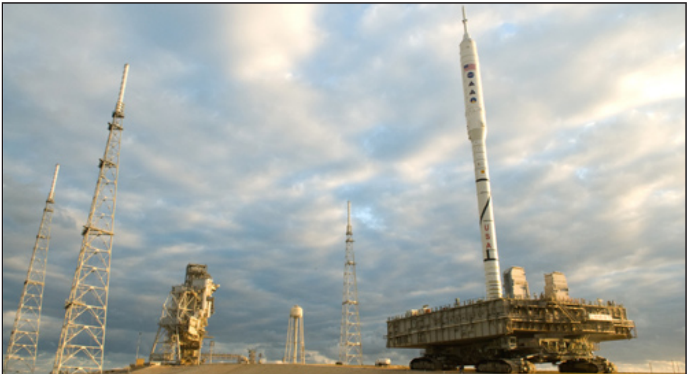
A crawler-transporter, traveling at less than 1 mph, takes the Ares I-X rocket to Launch Pad 39B at Kennedy Space Center.
