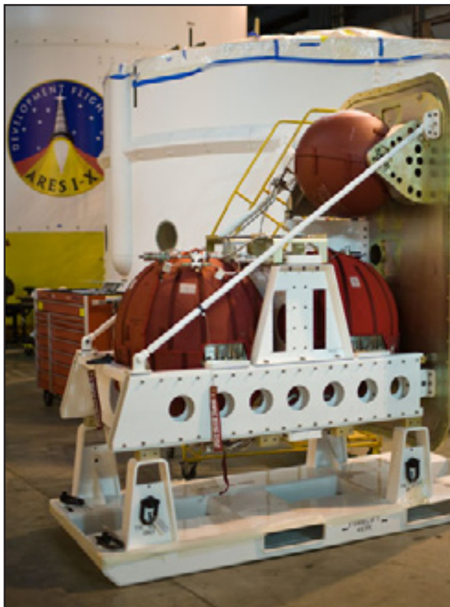
The Ares I-X roll control system module is revealed in Kennedy Space Center's Vehicle Assembly Building.
