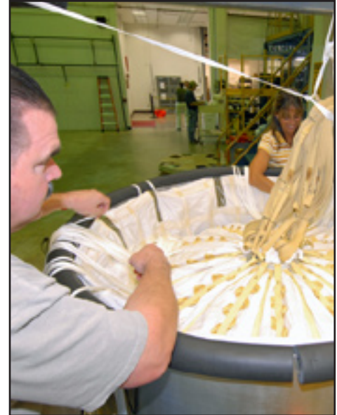
Workers pack an Ares I-X main parachute in Kennedy Space Center's Parachute Refurbishment Facility.
