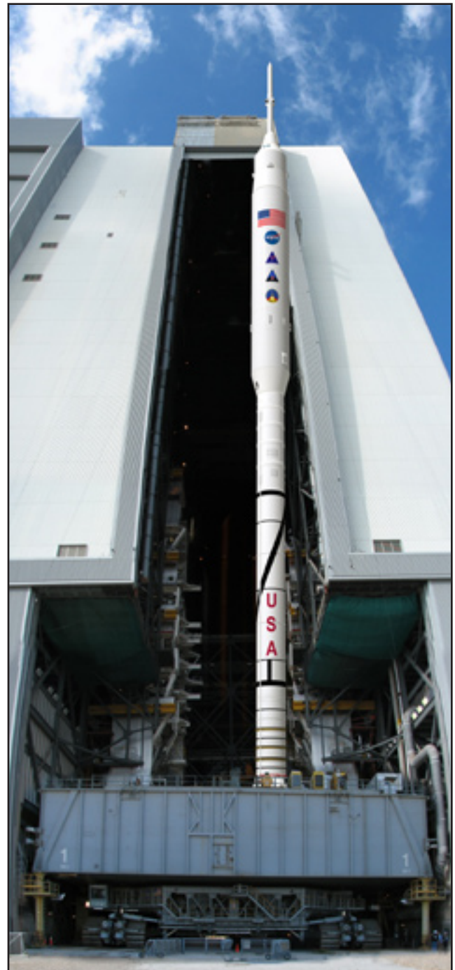
The Ares I-X rocket sits on one of NASA's giant mobile launcher platforms, MLP-1, which was modified for this flight test.
